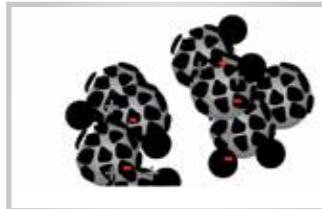
Re-agglomeration continues during grinding process
