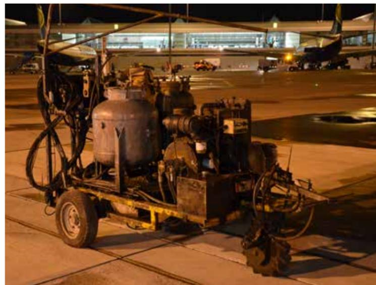
Fosroc Thioflex 555 rapid return to service joint sealant can be machine-applied to facilitate the best possible application rates. Parts A and B, in a 1:1 ratio, are fed along hoses to static mixers contained in the application lance, whereupon the finished product is mixed and delivered into the joint slot quickly and efficiently.
