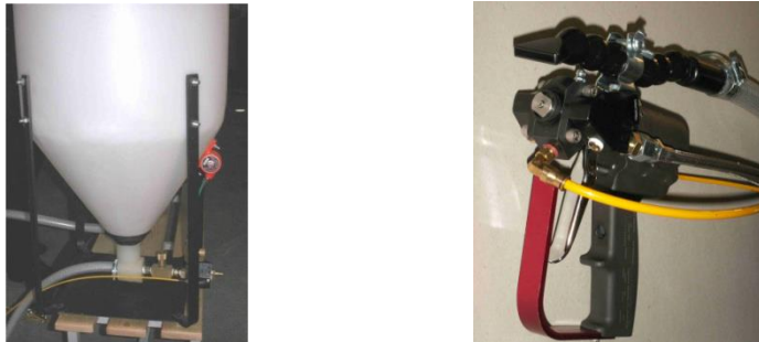
Fig: OL3K Drymix unit; storage (left) and modified spray gun with injector above spray nozzle (right)
