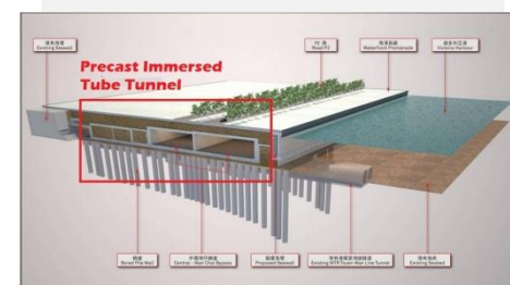
Precast tube tunnel over the existing MTR Tsuen Wan Line in position
